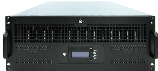
The FlexNAS TC 60BAYS ISCSI series RAID subsystem features high density disks capacity with ports on each controller to increase system efficiency and performance. It features high capability 1/10 Gigabit of expansion, with 60 hot-swappable SAS/SATA hard disk drive bays in a 19-inch 4U rackmount unit, scaling to a maximum storage capacity in the terabyte range.
